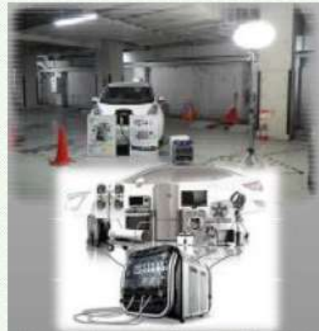
V2L System (Construction lighting) [Vehicle to Load]
